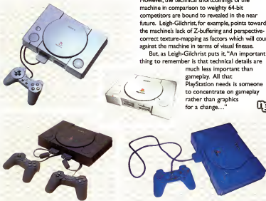
Sony has so far released four different versions of the PlayStation (from left): the standard gray model, the white Asia-only model (with enhanced MPEG playback), the programmable Yozora, and the development blue machine
